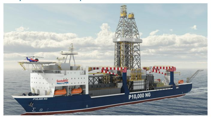
From the launch of the "Pelican" in 1972 GustoMSC has been involved in the design and construction of DP drill ships. During the 90's GustoMSC developed a new generation drill ship, capable of drilling in maximum 10,000 ft water depth. In 2007 the development of the P10,000 was taken a significant step further, enhancing the design ready to step into the next generation.
