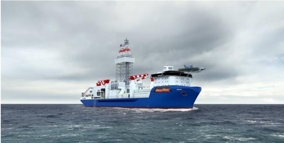
DUAL FUEL: GustoMSC has proposed designs that would add LNG fuel capacity to mobile offshore units, including deepwater drillships. Photo: GustoMSC
